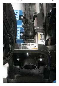
Then slowly thrust forward until the front (male) end of the pipe is in the jaws of the makeup wrench. Tighten the section of drill pipe onto the saver sub by locking the makeup wrench. Using forward rotation, rotate pipe until it is tightened to full drill rotation torque.
