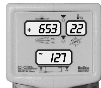
Locating Mode Showing Signal Strength, Transmitter Temperature, and Predicted Depth
