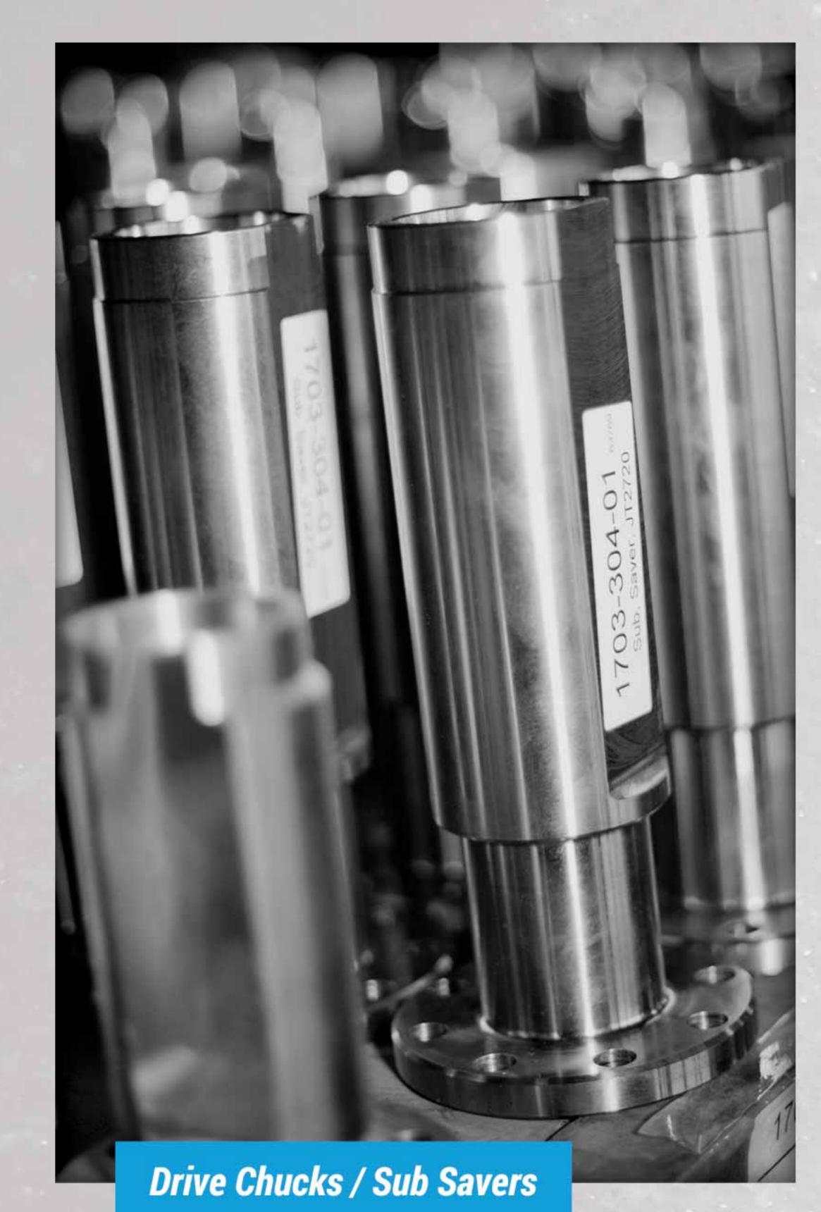
Available for all Vermeer®, Ditch Witch® and many other HDD rigs, our drive chucks and sub savers are machined to exacting standards from high strength alloy steel.
